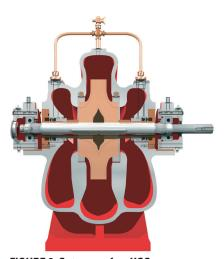
FIGURE 2. Cutaway of an HSC pump.
